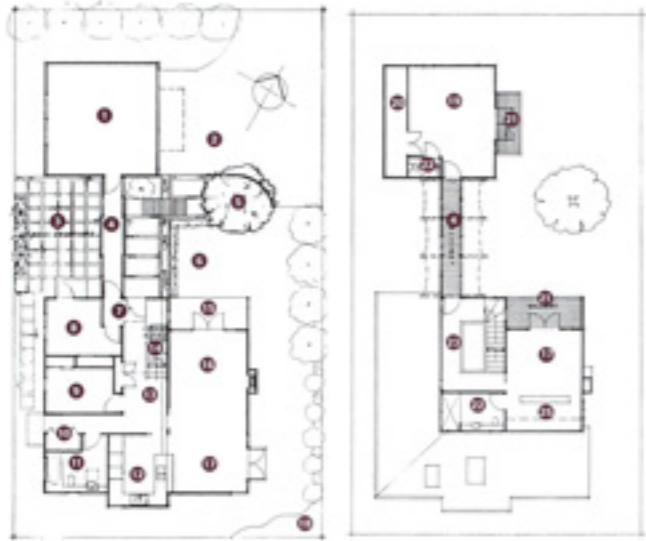
walkway (breezeway) with a tension membrane structure providing shelter overhead. The positioning of the boxes and walkway creates a series of sheltered gardens or courtyards enabling a place in the sun (or shade) to be found at any time of the day. Large sliding cedar doors open on both sides of the walkway to allow the sunshine and breeze to pass through and create a larger outdoor space as required.
